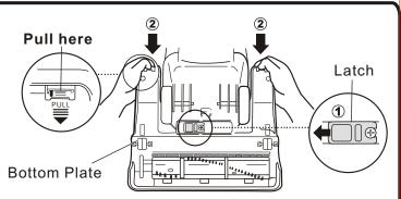
**3** Remove the bottom plate by pulling the tabs as illustrated.
